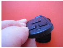
5. Press Silicone pad in till buttons are correctly positioned in respective holes of the plastic shell. Buttons should be positioned in cut outs of plastic shell as in the picture on the left.
